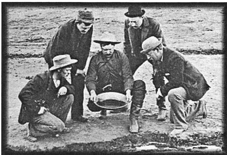
Miners pan for gold near a stream in Colorado. "Placer miners" try to shake out water and sand, leaving only gold in their pans.
