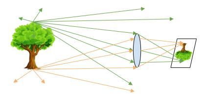
As the distance between the lens and the tree gets smaller, the image gets bigger but also farther away from the lens. To keep the image sharp the camera moves the light sensor farther away.
