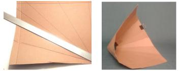
4. Glue aluminum to the surface of the cardboard, shiny-side up. Overlap edges. Try to keep the foil as smooth as possible. Some small bumps are not a problem.
