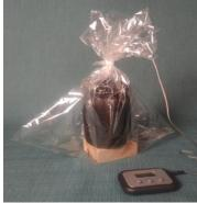
8. Place funnel in the banker's box. Put the jar in the center. Put the box in the sun and point the funnel towards the sun. On a warm day in April or May (in the Northern Hemisphere) near solar noon, the funnel should be able to pasteurize a pint of water in under 30 minutes.
