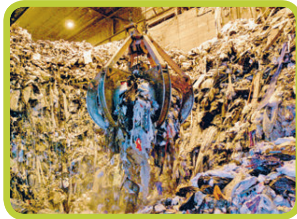
Garbage is lifted by a crane and placed into a hopper. Skip O'Rourke, Times
