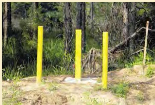
Monitoring wells ensure that groundwater is not contaminated.
