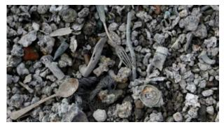
Magnets are used to recover ferrous metals, such as iron and steel, from the ash. Electrical currents called eddy currents are used to recover nonferrous metals such as aluminum and copper. The metals are then sold for recycling.
