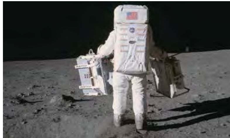
Astronaut Edwin E. "Buzz" Aldrin Jr., lunar module pilot, moves toward a position to deploy two components of the Early Apollo Scientific Experiments Package (EASEP) on the surface of the Moon during the Apollo 11 extravehicular activity. The Passive Seismic Experiments Package (PSEP) is in his left hand; and in his right hand is the Laser Ranging Retro-Reflector (LR3). NASA
