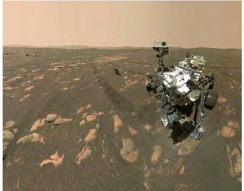
NASA's Perseverance Mars rover took a selfie with the Ingenuity helicopter, seen here about 13 feet (3.9 meters) from the rover in this image taken April 6, 2021. This image is made up of 62 individual images taken in sequence while the rover was looking at the helicopter, then again while it was looking at the camera, then stitched together once they are sent back to Earth. NASA
