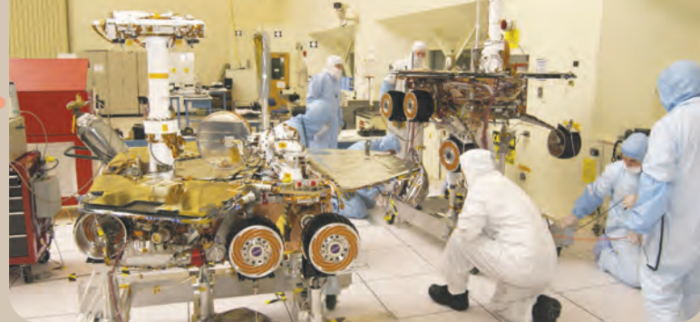
NASA's Spirit and Opportunity Mars rovers being tested. NASA/JPL-Caltech
